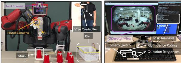
Fig. 3: Robot platform (left) and operator console (right).
