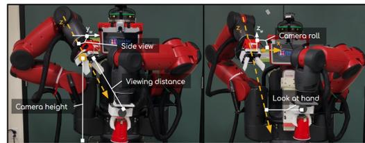
Fig. 2: Objectives for the autonomous camera control.
