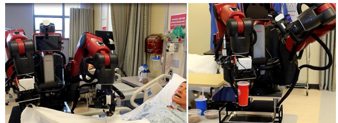
Fig. 1: Tele-nursing robots perform a variety of patient-caring tasks including cleaning and food delivery.
