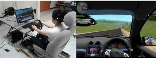
Fig. 3. A subject is driving in fixed-base simulation testbed within motion capture laboratory. (Left): Experimental setup. (Right): Screen capture of the driving simulator game
