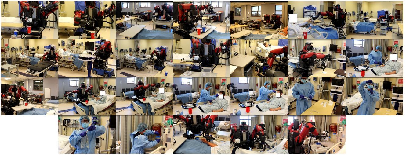
Fig. 4: Twenty-six nursing tasks (Table I) were performed in a simulated hospital room. Tasks not feasible for the robot are shown by nurse demonstration.
