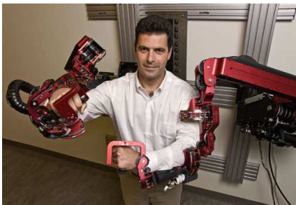
Fig. 1. The upper limb exoskeleton with seven DOFs, supporting 99% of the range of motion required to perform daily activities.
