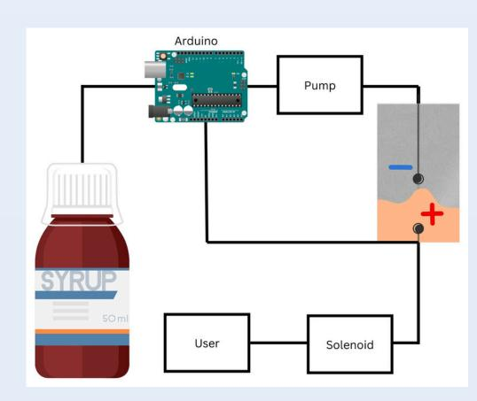
The current design utilizes an Arduino, peristaltic pumping motor, linear actuator, and solenoid. When the wire on the linear actuator comes into contact with the positively charged liquid, then the Arduino is triggered and the liquid stops pumping.
