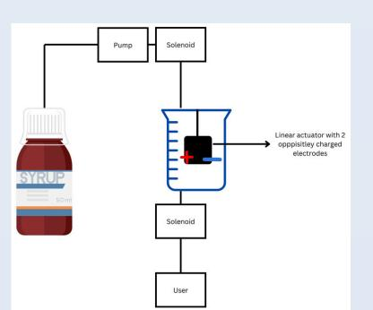
Used a linear actuator to indicate when height of specified volume was reached in known container.
