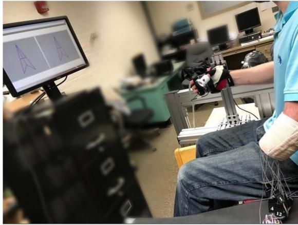
**Fig. 1.** Experimental apparatus. Subjects (limb-absent subject shown) sat in a chair with each able hand secured into force measurement devices, facing the computer screen which displayed a target and real-time force/moment feedback.
