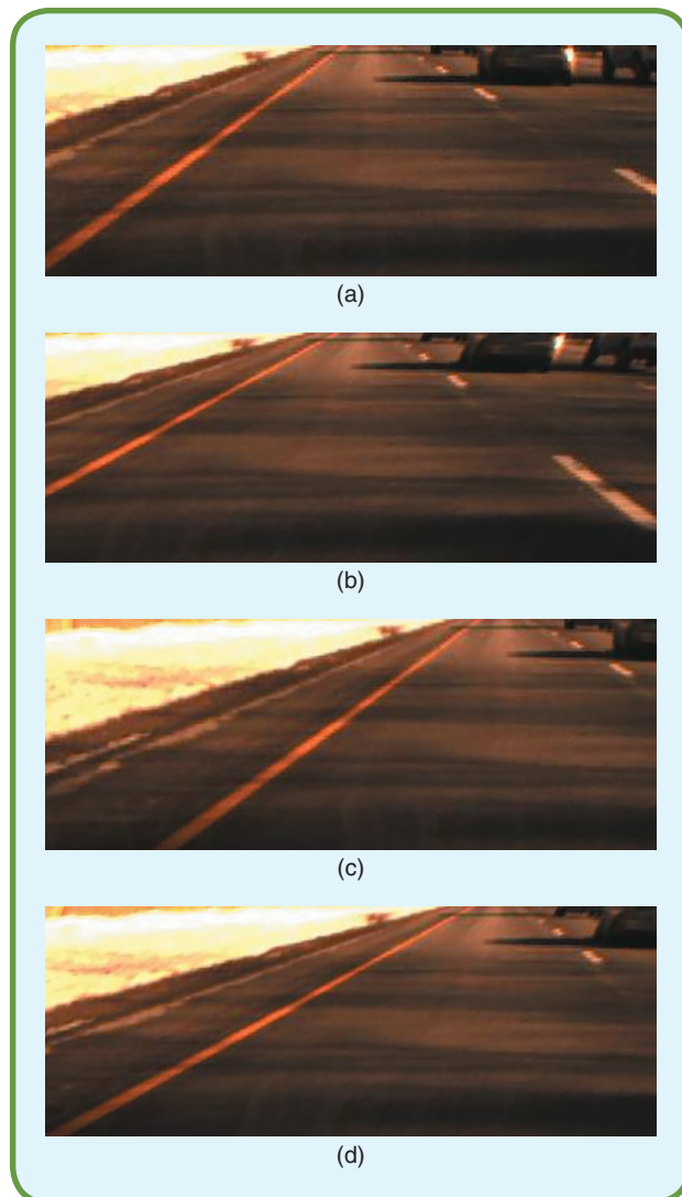
FIG 12 Example of original image and augmented images given arbitrary vehicle poses. (a) Original image. (b) Augmented image as if the vehicle is shifted right by 0.5 m. (c) Augmented image as if the vehicle is rotated left by 7 degrees. (d) Augmented image as if the vehicle is shifted right by 0.5 m and rotated left by 7 degrees.
