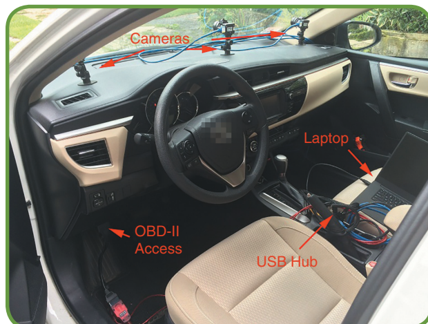
FIG 10 The data collection system including three forward facing cameras, a USB hub, a laptop computer with access to OBD-II port.
