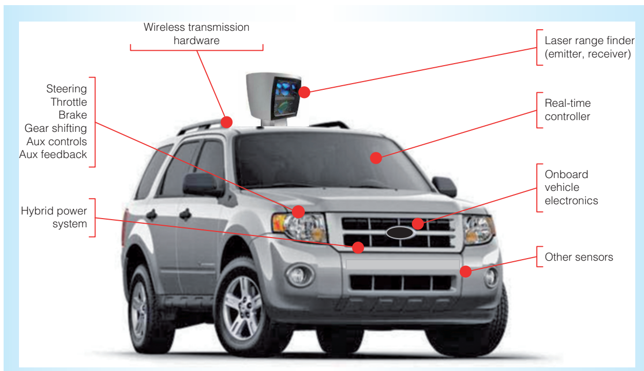
Figure 2. An autonomous automotive system with an array of sensors, embedded computing devices, and communication systems. One or more of these components could be compromised in a physical security attack.
