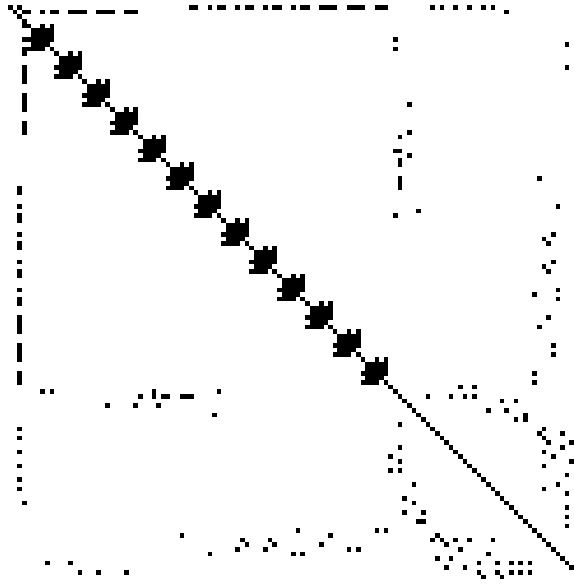
Figure 2. Jacobian matrix sparsity pattern corresponding to the circuit 'bgatt'
