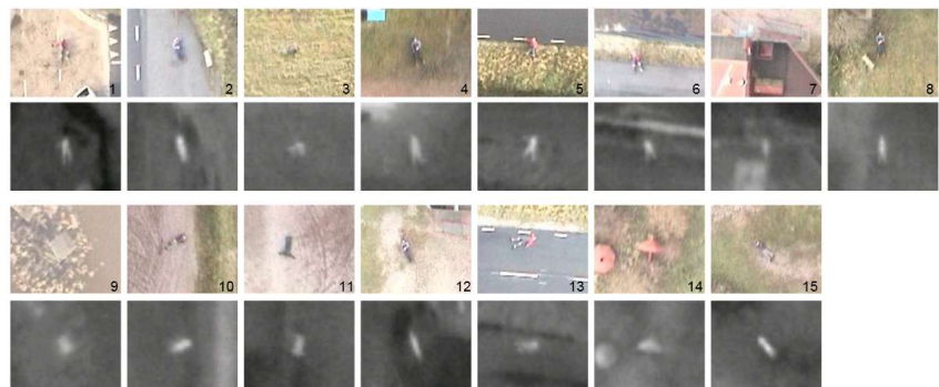
Fig. 6. Images of classified bodies. Corresponding thermal images are placed under color images.
