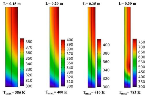
Figure 2. Three-layered scenario (Figure 1) with material parameters from [9]: steady-state temperature profiles for different lengths of the channel; incident power density  $4,200 \text{ W/m}^2$ .
