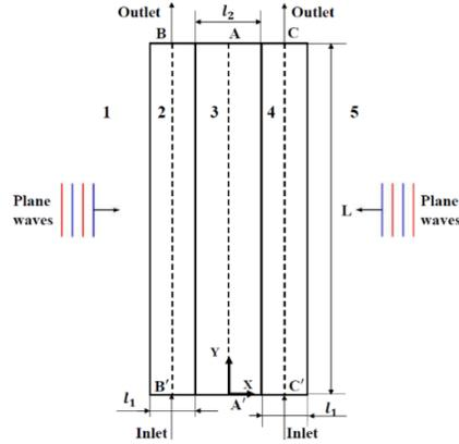
Figure 1. Triple-layered geometry subjected to symmetric MW irradiation; media 1 and 5 are free space, media 2 and 4 are lossless fluid, and medium 3 is lossy dielectric;  $L$  is the length of channels.
