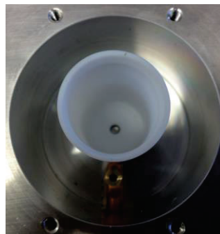
Figure 2. Internal view of the cylindrical cavity of the SAIREM's reactor MiniFlow 200SS system.
