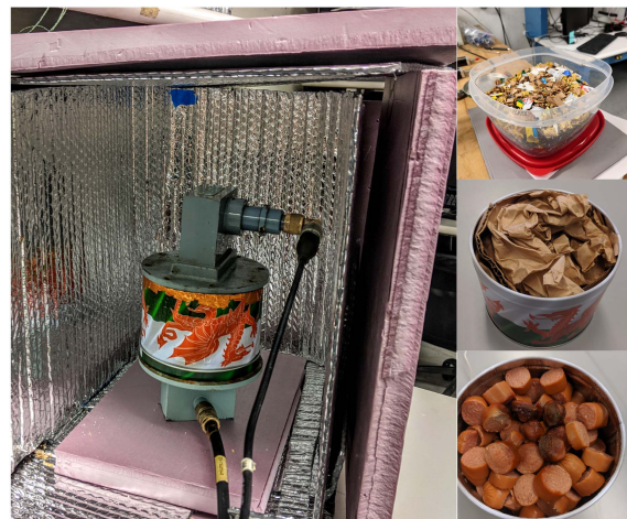
FIGURE 11. Photograph showing the 1.4ℓ heating cavity with two waveguide feeds, and with 2.75-cm thick thermal insulation. Several photographs of different waste mixtures are also shown: (top) medium \epsilon_r mixture; (center) paper loading; and (bottom) meat loading after 20 minutes of heating.
