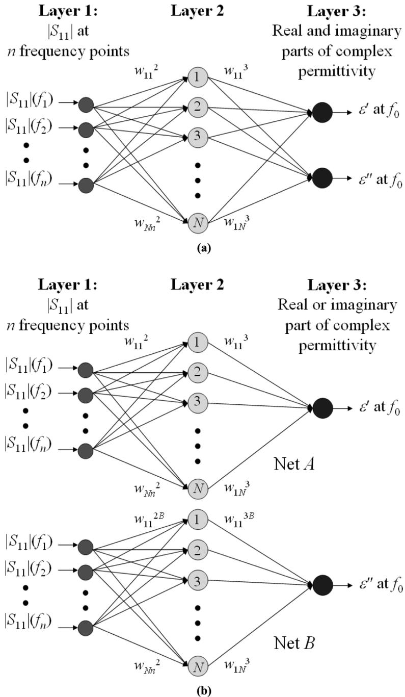
**Figure 2.** MLP networks for the one-port system: (a)  $n$ - and (b)  $2 \times n$ -input architectures
