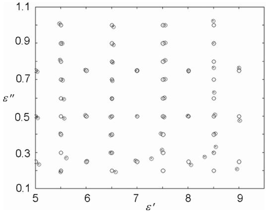
**Figure 5.** Complex permittivity reconstructed with the  $2 \times n$ -input MLP with  $N_A = N_B = 10$ : circles and crossed circles mark the test data and the actual responses, respectively
