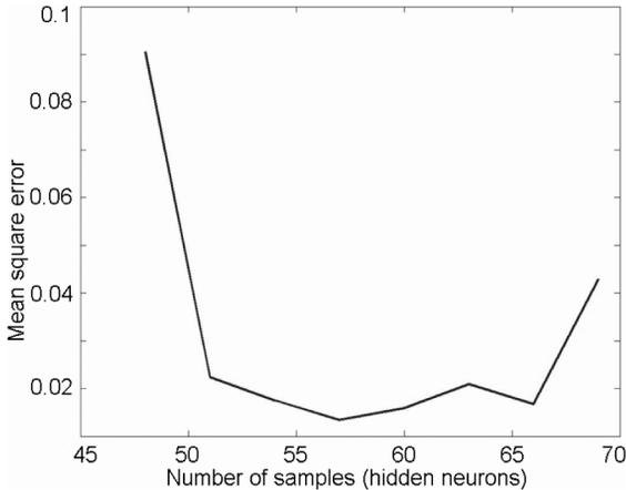
**Figure 6.** MSE of the 2-input RBF with the number of training samples from 48 to 69 with step 3
