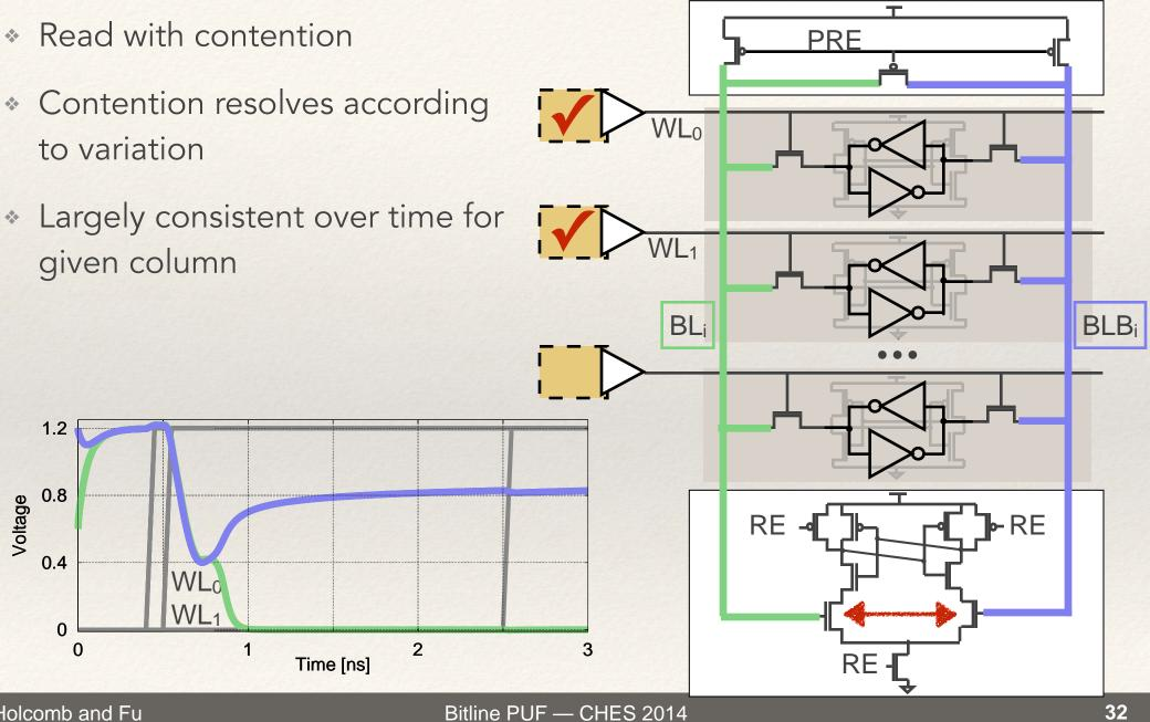
Read with contention \* PRE Contention resolves according \* WL<sub>0</sub> to variation Largely consistent over time for VL 1 given column **BLB**<sub>i</sub> BL 1.2 0.8 Voltage RE RE 0.4 M W/ 0 2 0 1 3 Time [ns] RE
