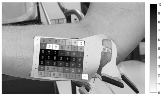
Figure 1: A visualization of the output from the OptiMyo system on a subject's extensor muscles. Darker sections reflect a higher (better) score.
