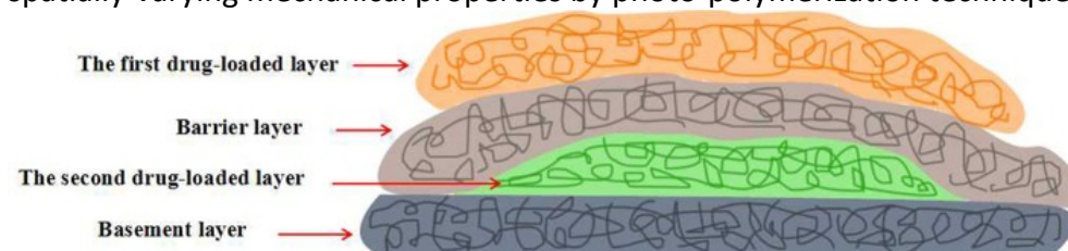
Figure 6: Schematic representation of four-layered hydrogels with time-programmed combination release behavior by sequential electrospinning technique.
