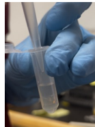
Figure 2. Collecting samples by pipetting the surrounding PBS. Within the PBS, there is released dextran. To measure it, the solution will be pipetted into a black-well plate.
