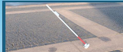
Figure 6: Prototype 4- created with ASA + ABS Plastic
