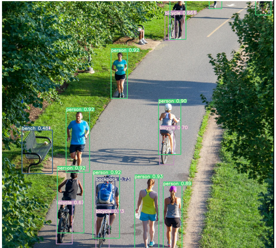
Example of object detection, done with YOLOv7. Note the bounding boxes and confidence levels
