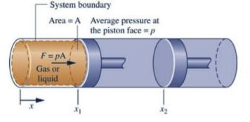
During the process, the gas exerts a normal force on the piston, F = pA, where p is the pressure at the interface between the gas and piston and A is the area of the piston face.
