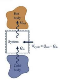
► As for the refrigeration cycle, the energy balance reads
