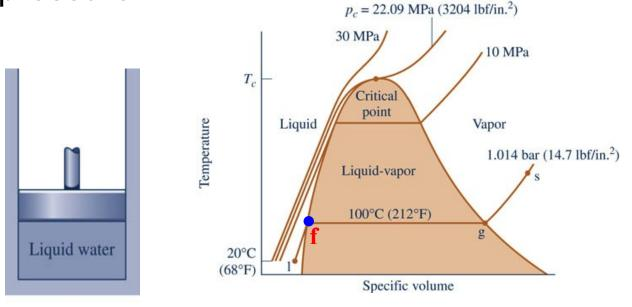
When the system is at the saturated liquid state, additional heat transfer at fixed pressure results in the formation of vapor without change in temperature but with a considerable increase in specific volume as shown by movement of the blue dot.
