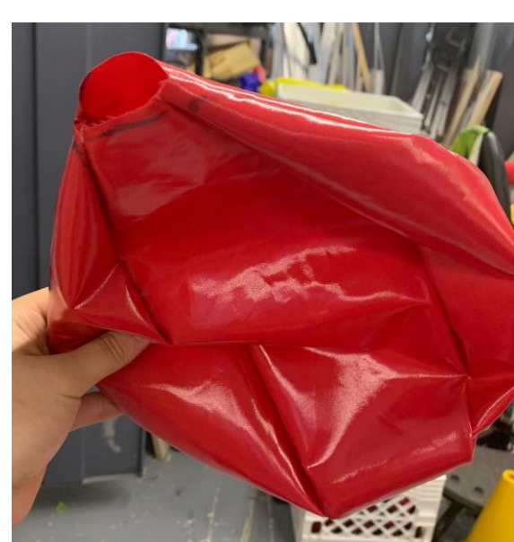
Figure 4. Airbag after sealing seams . One of the airbags after sealing of seams and inversion of the fabric
