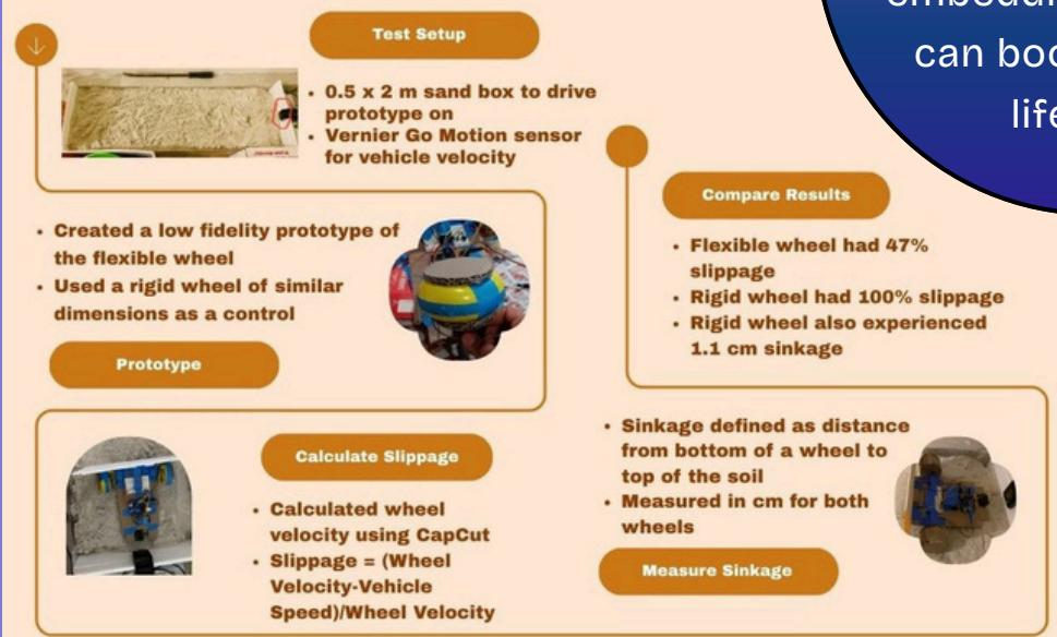
Rover wheels that autonomously adjust their geometry based on a rover's embedding condition can boost mission lifetime.
