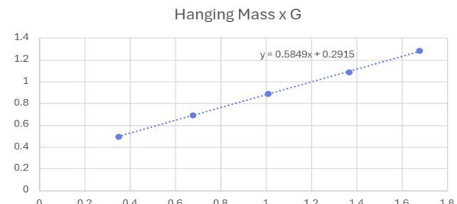
The slope of the graph is slightly higher than the measured mass of the system. This means that the actual acceleration would be a little lower than the theoretical acceleration. The main source of this difference is the presence of friction between the wheels of the cart and the track that is ignored in the calculations. Other sources could include a slight upward inclination in the ramp and friction around the axle of the pulley.
