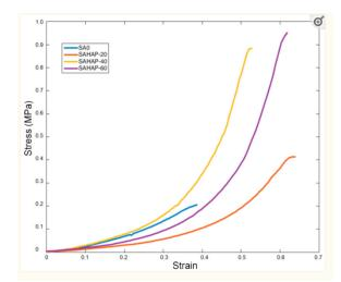
**Table 2:** Shows a stress-strain curve in a test on the effects on the mechanical properties of alginate with the addition of hydroxyapatite (Sánchez-Fernández et al., 2021). This curve shows the material's behavior when under extreme force and focuses on the part of the graph where each line is linear since stress is linearly proportional to strain. With the slope being Young's Modulus, this graph also shows the elasticity of each concentration.
