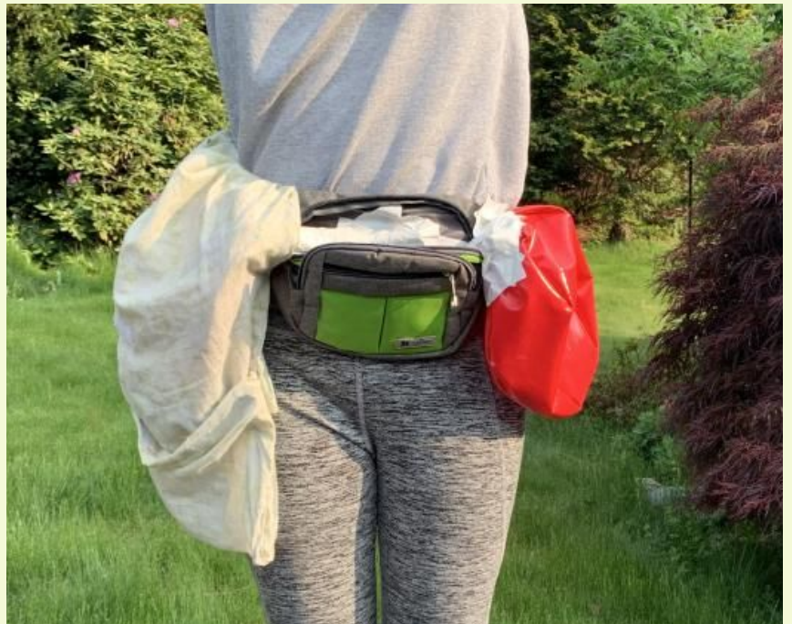
Figure 2: TrustFall while on an individual and half of it covered. This image contains the TrustFall device where one half of it is covered by fabric. The airbag on the other hip is unobstructed.
