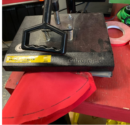
Figure 9: Sealing Airbag. A T-shirt press was used to heat seal the fabric seams. Only the seam allowance is heat sealed.
