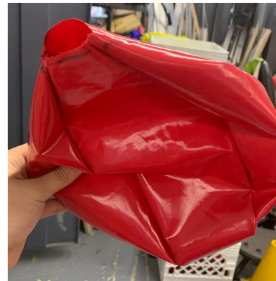
Figure 11. Airbag after sealing seams and inverting. One of the airbags after sealing of seams and inversion of the fabric
