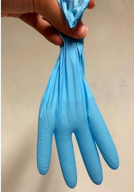
Figure 14. Glove filled with water. The glove filled with water which will be attached to the inlet port of the valve.
