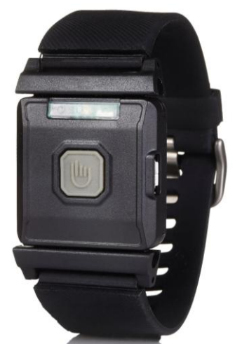
Figure 10: TouchPoint Wristband Competitor . Tracks heartbeat and other physical identifiers to identify an episode.
