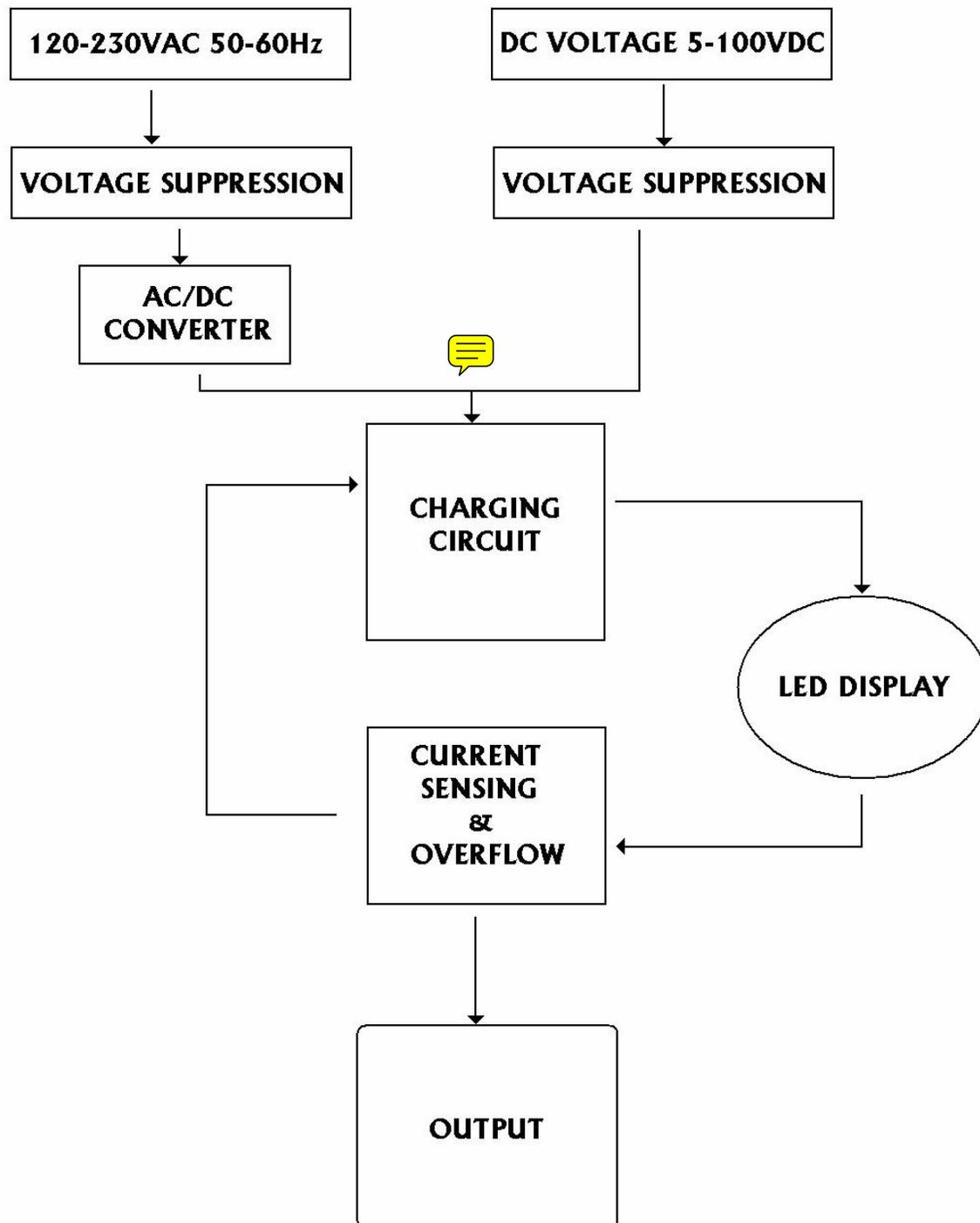
Figure 1: System Block Diagram for the Universal Car Battery Charger
