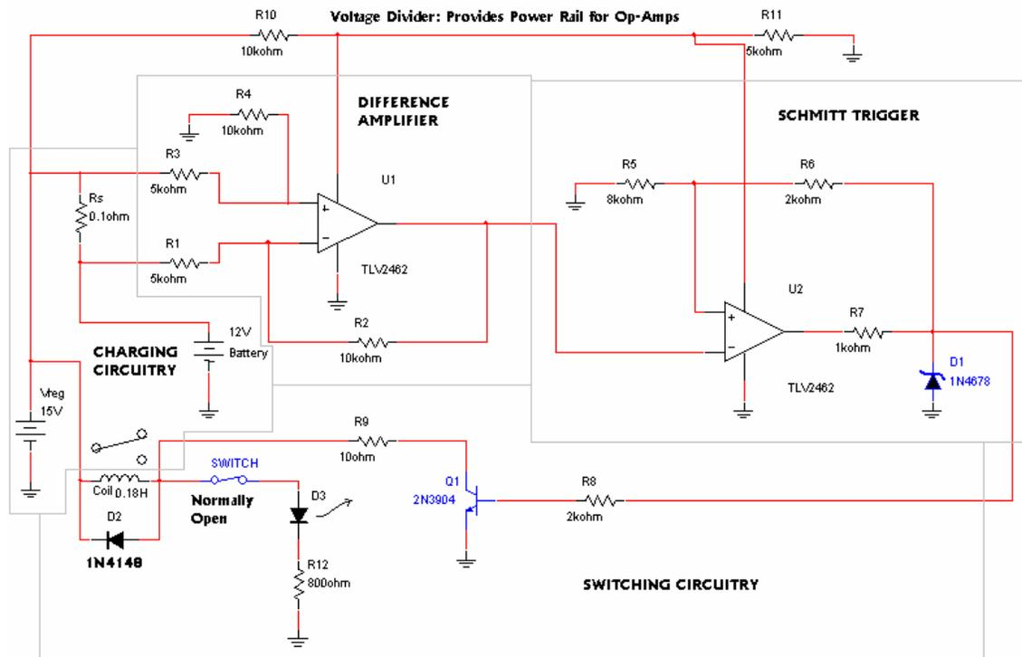
Figure 5: The Overcharge Protection Circuit
