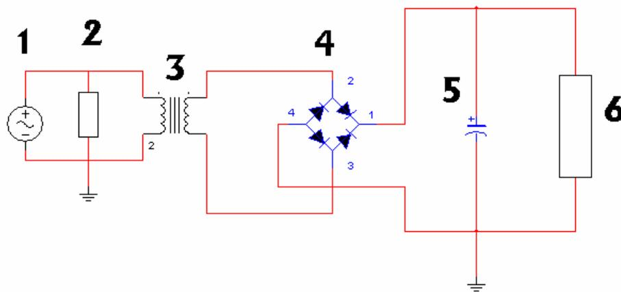
Figure 3: Revised AC/DC Conversion Circuit
