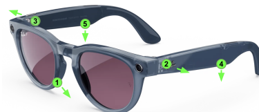
Fig. 1: Ray-Ban Meta microphone positions, channel numbers and porting directions (indicated by green arrows).
