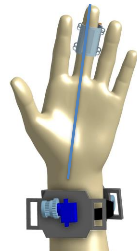
Figure 3. Two cords (blue line) pull back the top and back of finger detected during tremor activity. Springs are not used to force modulation. (Golji et al., 2026)
