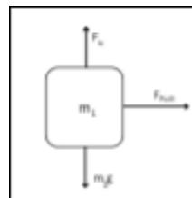
The free body diagram in Figure 1 shows the forces affecting on the cart in our experiment.
