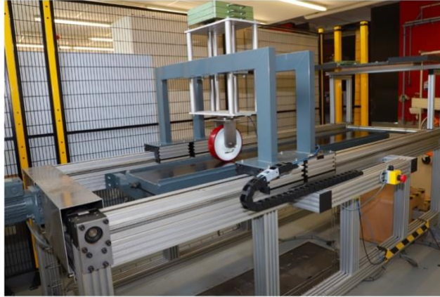
Figure 1 shows the equipment used to measure the resistive forces for a single wheel under controlled, uniform motion. This system eliminated energy losses not related to wheel/floor contact, providing the input data needed to calculate the corrective forces for the model.
