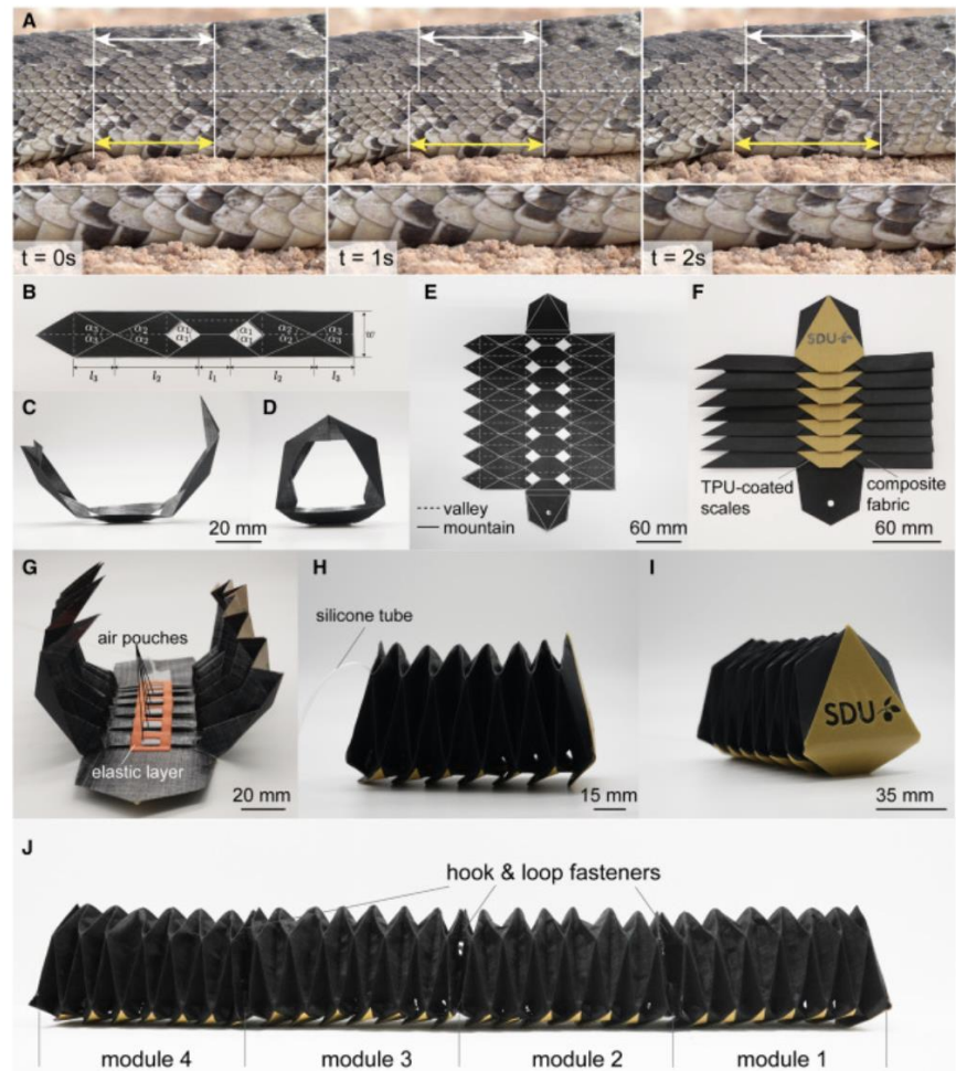
Figure 1. Depiction of snake inspired robot compared to a puff adder snake during rectilinear locomotion.
