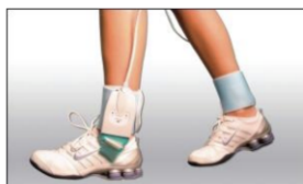
Figure 3-4: In shoe systems (Novel Pedar, Tekscan F-scan), with flexible insoles and tethered or belt mounted electronics, highlighting benefits (portability, real-world gait) and drawbacks (slippage, lower spatial resolution)
