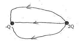
(b) The figure to the right above shows a positive charge 2Q and a negative charge –Q a certain distance apart. Draw at least three field lines passing through both charges, and also indicate the arrows on them. (5pts)
