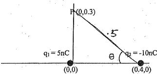
(a) Calculate the components (E<sub>1x</sub>,E<sub>1y</sub>) of the electric field at P due to the charge q<sub>1</sub>.
