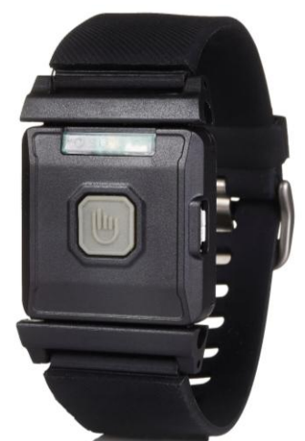
Figure 10: TouchPoint Wristband Competitor . Tracks heartbeat and other physical identifiers to identify an episode.
