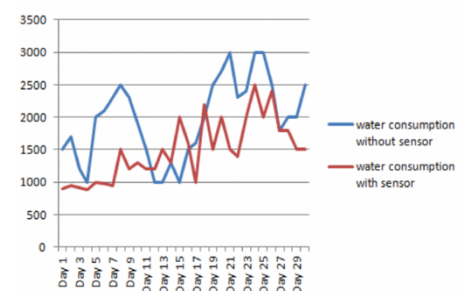
Figure 3: Graph shows us the red line, which is the water consumption with a sensor being under the blue line, which did not have a sensor (Taneja, & Bhati, 2017)
