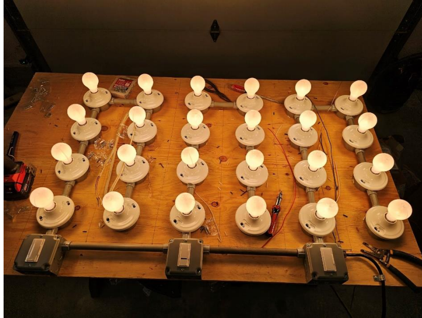
Figure 4. The array of 24, 72W halogen light bulbs used to provide radiant energy and heat to the PV.
