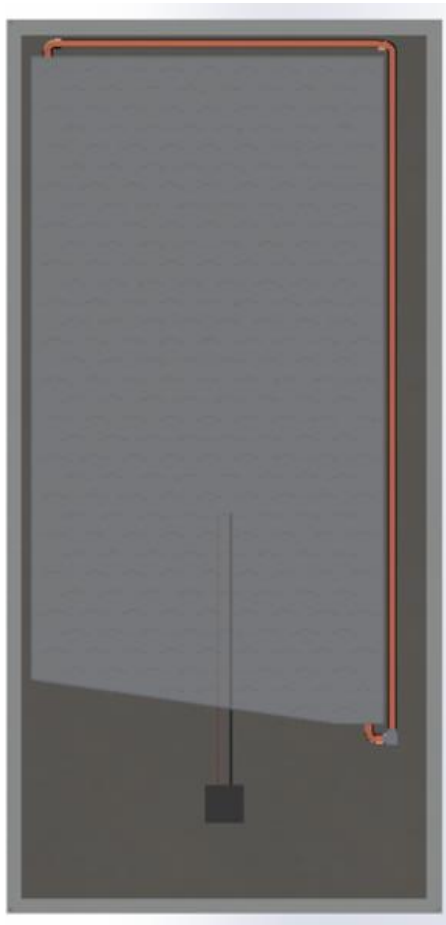
Figure 7. SolidWorks model of aluminum water block on the rear of a PV. An intake can be found at the top of the PV and an exhaust at the bottom of the PV.
