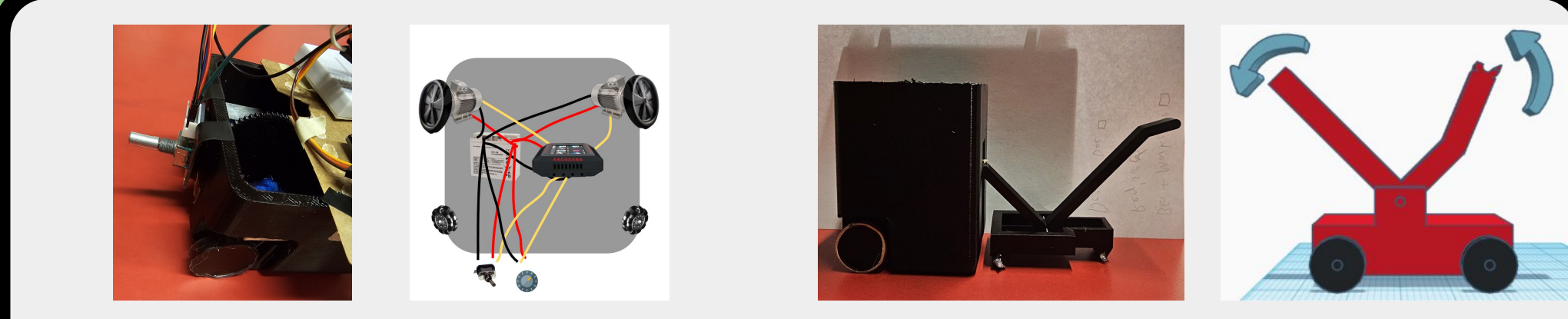
Figures 1, 2: 3D printed trash can with two servo motors controlled by an Arduino UNO. The system features a knob to change the rotational velocity.
