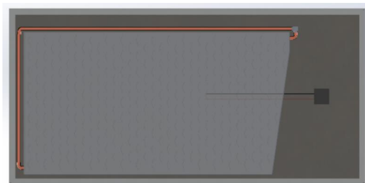
Figure 2. SolidWorks model of aluminum water block on the rear of a PV (iteration 1). The right side represents the lower half of the PV.
