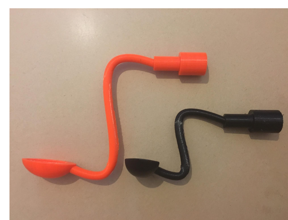
Figure 6: A comparison of the two lengths of the spoon neck that were tested
