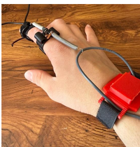
Figure 1. Spring-system is attached between the finger and wrist to automatically reduce tremor-like oscillations (Golji et al., 2026).
