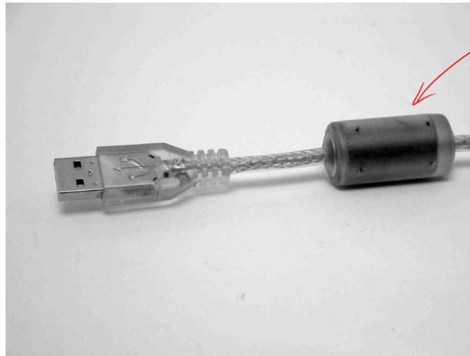
Figure 5-32: Ferrite core used on a USB cable to suppress radiated emissions
