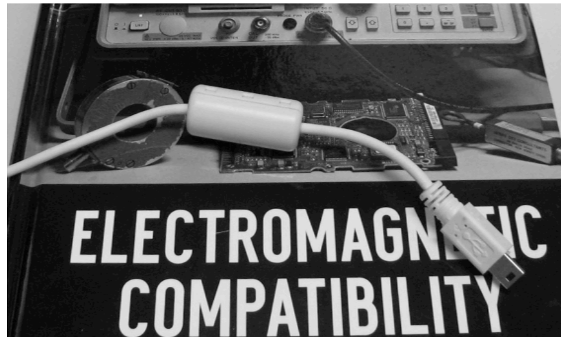
Figure 3-43: An easy way to place a common-mode choke in the circuit is to wind both conductors around a torodial magnetic core. A coaxial cable may also be used in place of the conductors shown
