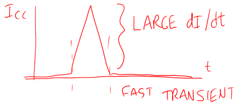
Figure 11-2: Transient currents produced when a CMOS logic gate switches
