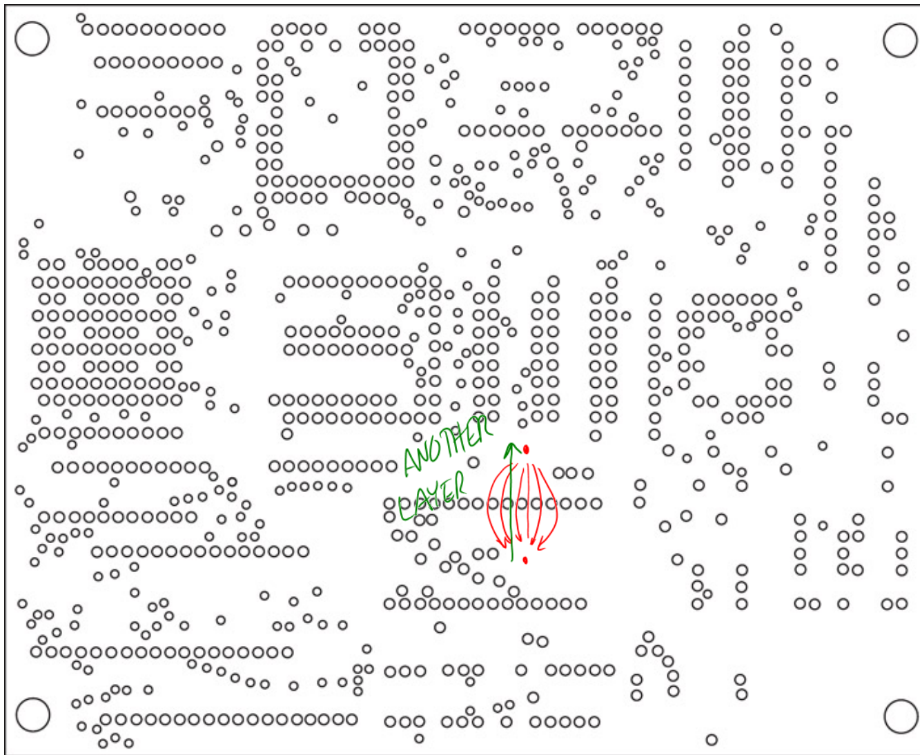
Figure 10-6: Typical printed circuit board ground plane
