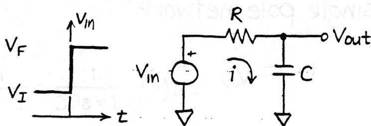
First order differential equation for  $V_{out}$
