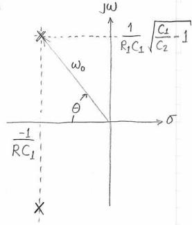
We still have R and  $C_1$  or  $C_2$  as free parameters, with the constraint that  $C_1 > C_2$ .
