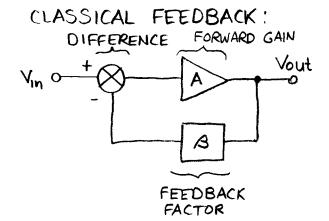
B: "FEEDBACK FACTOR" FRACTION OF Vout FED BACK TO V\_
