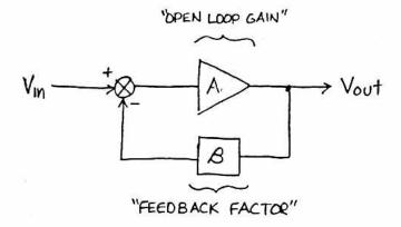
Equation around loop; A finite LOOP GAIN"
